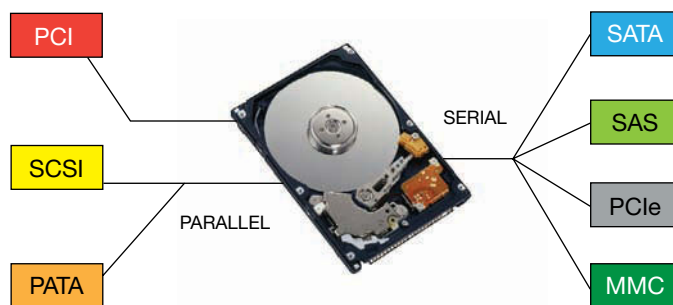
Figure 1 The older, high-power interfaces, including PATA, SCSI, and PCI, had multiple-data-pin, wide-cable interfaces. The new interfaces, including SATA, SAS, and PCIe, all have high data rates with only a few active pins.
