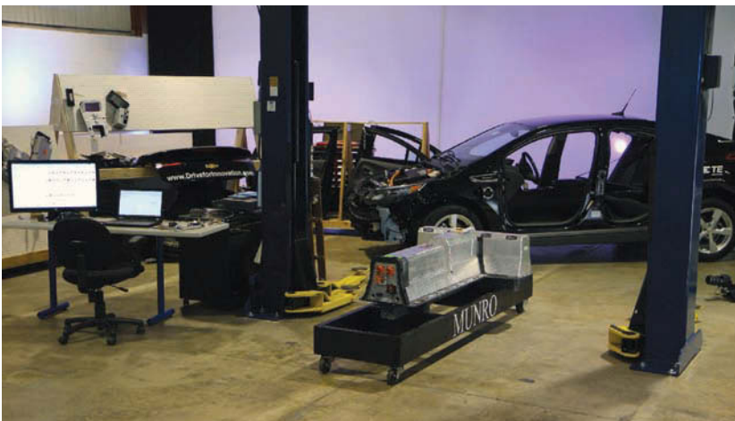
Figure 1 The 375-lb (170-kg) lithium-ion battery pack is the heart of the Volt. The vehicle’s systems and software maintain the battery pack’s health for a long service life (courtesy Munro & Associates).
